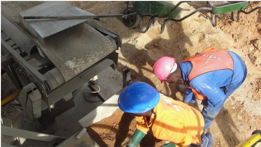
Figure 6: the sand and cement mixture is being prepared for producing first blocks of bricks.
