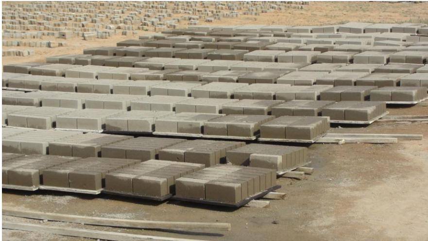
Figure 10: Wet, newly produced bricks packed on pallets for drying.
